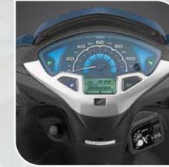
**DIGITAL ANALOG METER WITH ECO SPEED INDICATOR**
